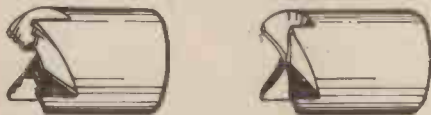
Fig. 2.—Hollow cutters require special treatment as regards backing off as will be seen from the sketch.
