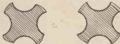
Figs. 7 and 8.—(Left) Overcoming a weak tap by relieving the taps of the thread and (right) a tap with the threads relieved at the root, crest, and flanks.
