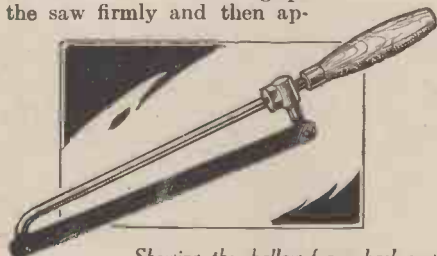
Showing the shallow frame hack-saw which is ideal for work where limited space makes it impossible to use a standard hack-saw.
