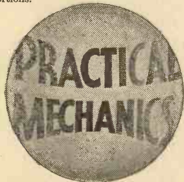
Diagram explaining the fault known as spherical aberration.
