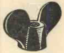
Fig. 5.—A typical wing nut.
