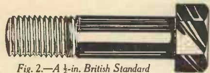
Fig. 2.—A 1/2-in. British Standard Fine bolt.
