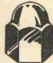
Fig. 4.—This type of nut is known as a cap nut.
