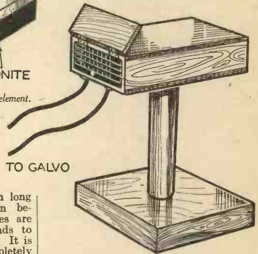
Fig. 5.—Showing the completed instrument suitably mounted on a wooden stand.
