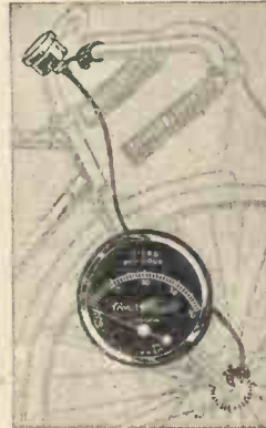
The Cooper Stewart speedometer for fitting to bicycles, which was described on page 335 of last month's issue.
