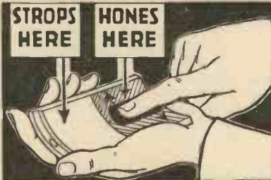
Showing the method of using the "Newstrop." This device can be used to hone or strop safety-razor blades.
