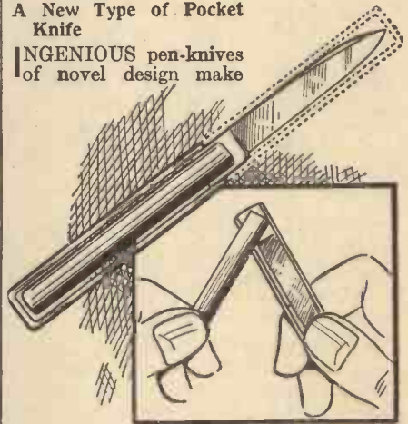
An ingenious one-blade pocket knife which is easy to open, and the blade is held rigid when the knife is in use.
