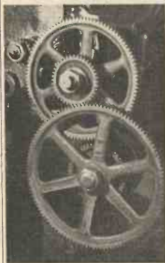
Fig. 2.—A compound train. The gear behind the lead-screw wheel is used as packing.
