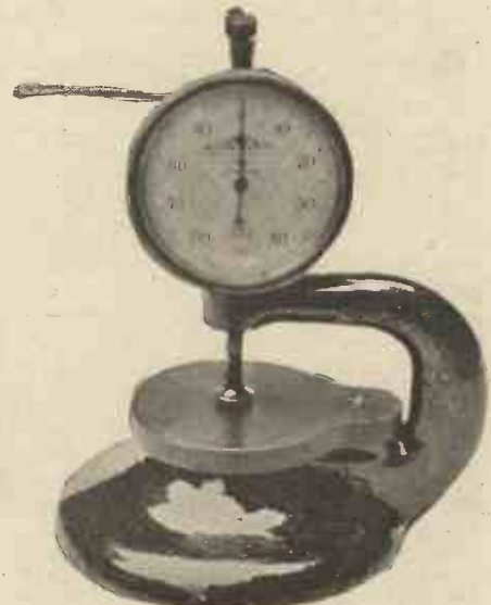
Fig. 4.—Even this job did not defeat the skill of the modern welder. Here is the repaired gauge; it functioned perfectly.
