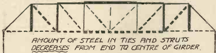
Fig. 12.—An outline of a steel framed girder, showing the compressional members in solid lines and the tensile members dotted. Note the varying amount of steel required in the various members.
