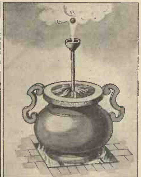
Fig. 2.—A steam turbine invented 2,000 years ago by Heron of Alexandria, and (right) a ball suspended in a column of steam.
