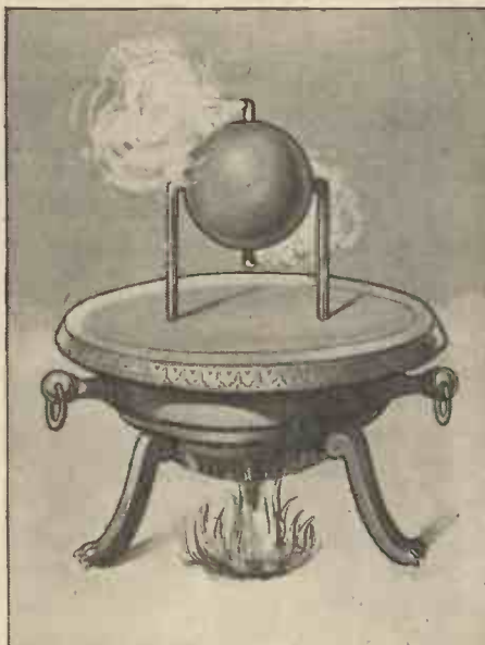
Fig. 2.—A steam turbine invented 2,000 years ago by Heron of Alexandria, and (right) a ball suspended in a column of steam.
