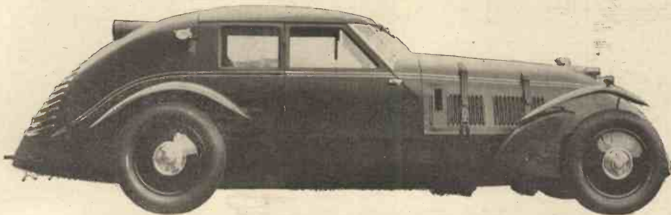
This impressive-looking saloon was built experimentally to test out the possibilities of the Diesel engine for high-speed purposes. Driven by Captain G. E. T. Eyston, it achieved a speed of over 100 m.p.h. on Brooklands.
