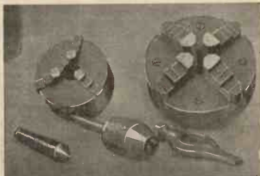
Fig. 2.—Showing carriers of drop-forged steel, a drill chuck for the tail stock, a conical lathe centre, and three- and four-jawed chucks.
