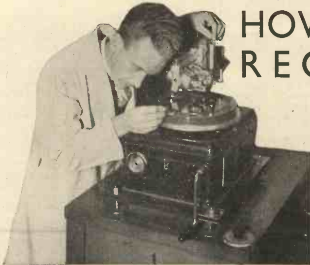
A recording engineer examining a wax recording immediately after a record has been made.
