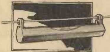
An aluminium line and surface level suitable for laying brickwork, pipe-lines, etc.
