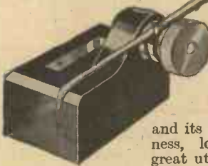
Details of the midget scribing block.
