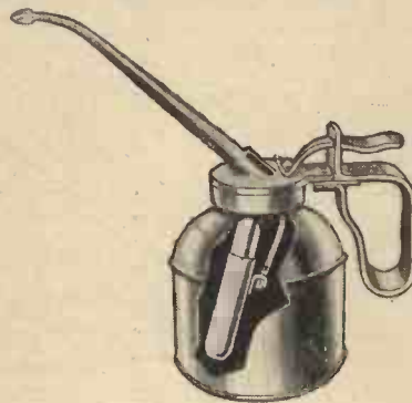
A broken view of the "Wesco" oil-can showing how the oil is ejected.
