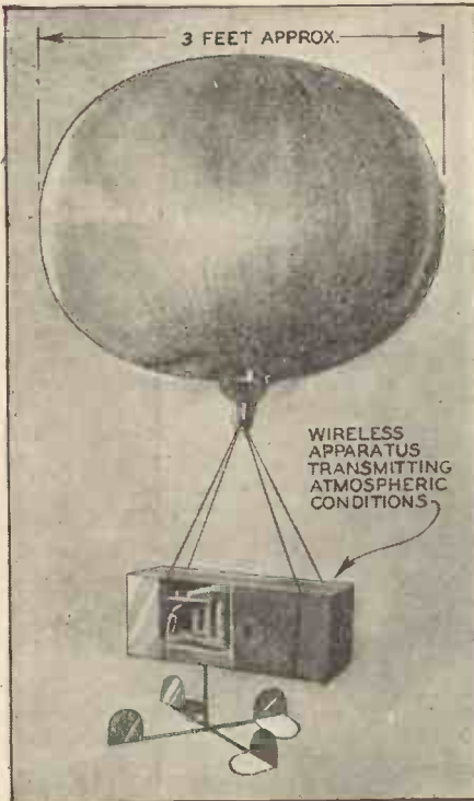
How some of the stratosphere explorations are conducted. Note the wireless transmitting apparatus.
