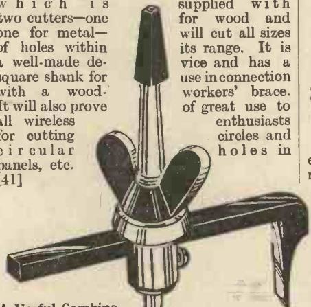
A handy trepanning cutter that can be adjusted to cut any size hole within its range.
