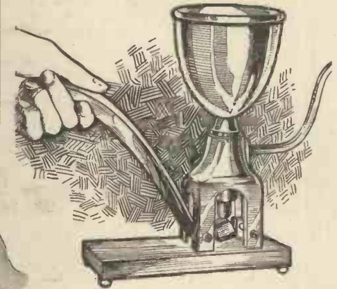
A super cream machine, which makes the finest cream from butter and milk.
