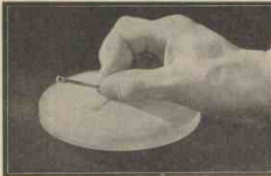
Fig. 2.—A tiny lens stuck on a "peg" to handle it for polishing.
