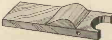
Fig. 3.—The trigger for stopping the flow of air in the air pipe.
