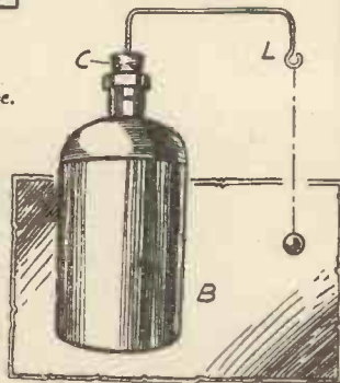
Fig. 4.—A simple stand for suspending pith balls, etc.
