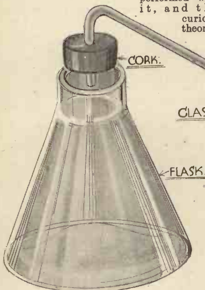
Fig. 3.—A cork is bored to accommodate the tube as shown.
