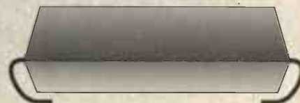
Fig.4. J lead package.
