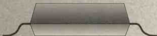
Fig.4. Gull wing package.
