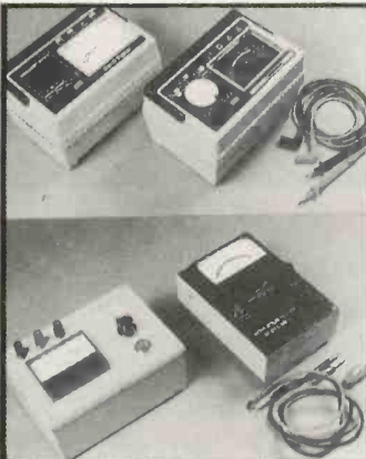
Photos: (Top) the genuine Megger instruments, (below) the potentially lethal fakes.
