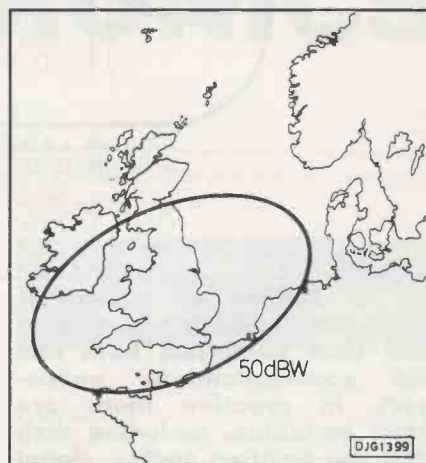
Fig. 5. Coverage of a satellite transponder beam or 'footprint', is shown by contour lines like this. Here the line encloses an area of signal strength corresponding to a beam eirp of 50 dbW (100 kW). Other such contour lines outside this one would show how the eirp tails off at the outer edges of the coverage.
