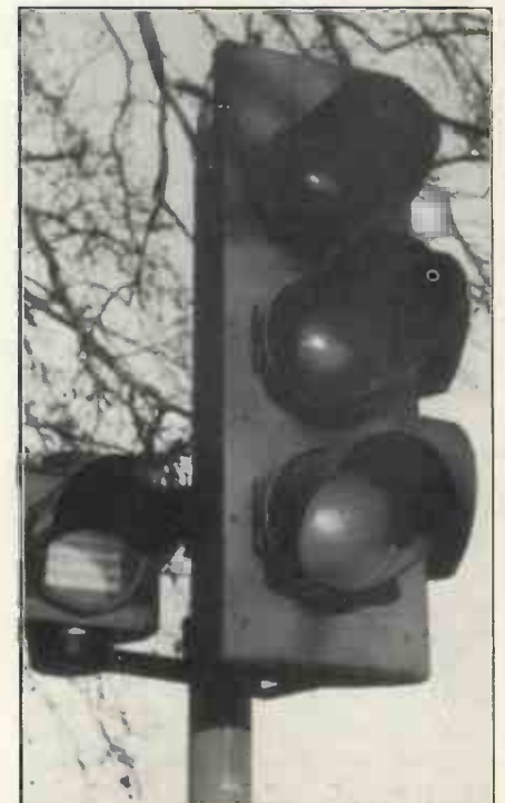
Infra-red beacon mounted on traffic lights
