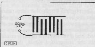
Fig.4. Leaving out the middle of the transducer finger in this manner considerably reduces the mechanical loading on the crystal.
