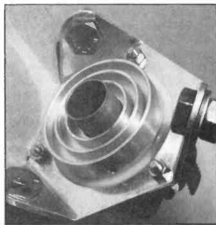
Fig. 4. The scalar feedhorn for the 11 Ghz band.
