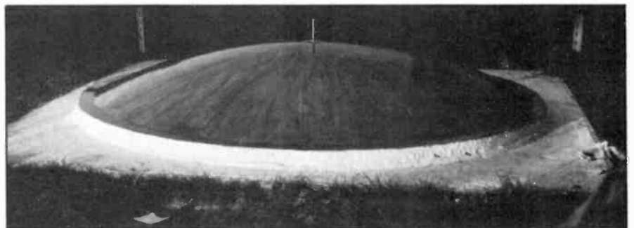
Fig. 2. A high gloss finish is obtained by coating the mould with 'Shellac' or a similar varnish.
