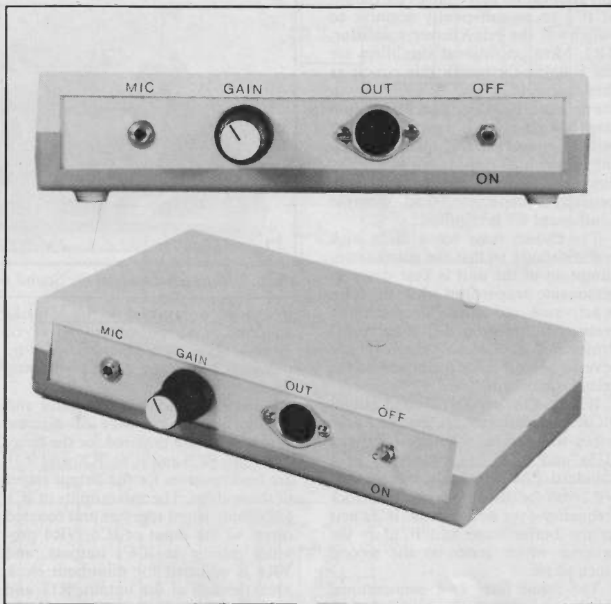
Photo 3. Front panel and case details of the Sound Activated Switch
