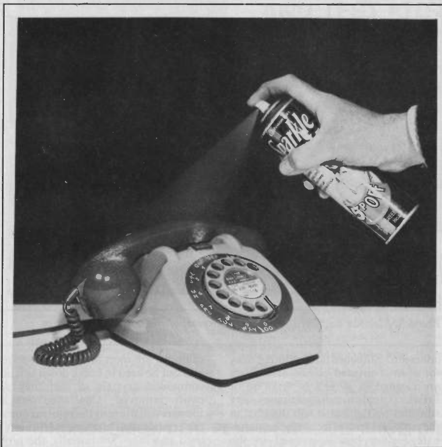
Photo 1. Silicone contamination, the hidden menace, caused by innocent use of spray polish
