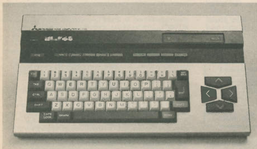
A home computer (above) is an example of a microprocessor system. The machine shown is based on a standard 8-bit micro
