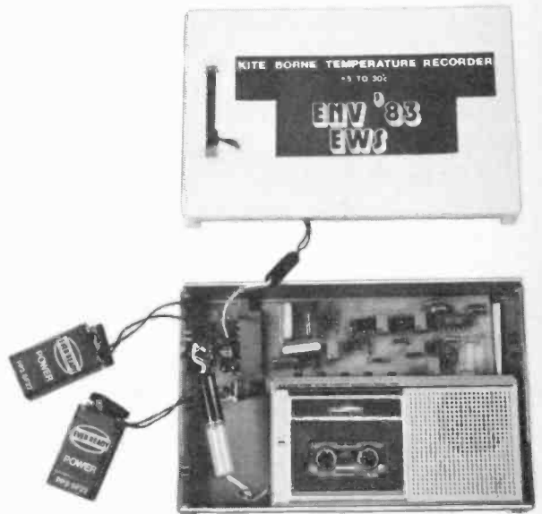
Fig. 1. Voltage-to-Frequency converter in the guise of temperature sensor. This circuit produces temperature related frequencies in a range suitable for domestic cassette recorders
