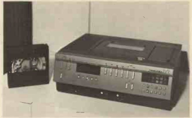
The LVR system from Toshiba employs a continuous tape loop with the audio and video encoded together.
