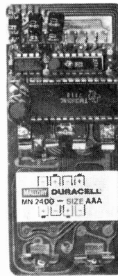
Rear view of the calculator showing the i.s.i. main chip and display driver
