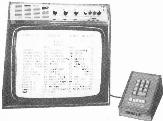
A TV set displaying an Oracle index page. The small unit is the decoder
