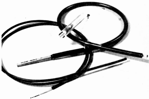
Arrangement of 3 light guides. The Crofon 64 filament guide in plastics and two "mares" tails in glass. Notice the polished ends
