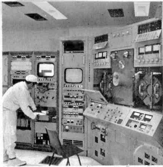
General view of the Electron Beam Recorder in use at the EVR processing plant. The special clothing worn by the operators together with the filtered air supplied maintains the high degree of cleanliness required in the manufacturing process
