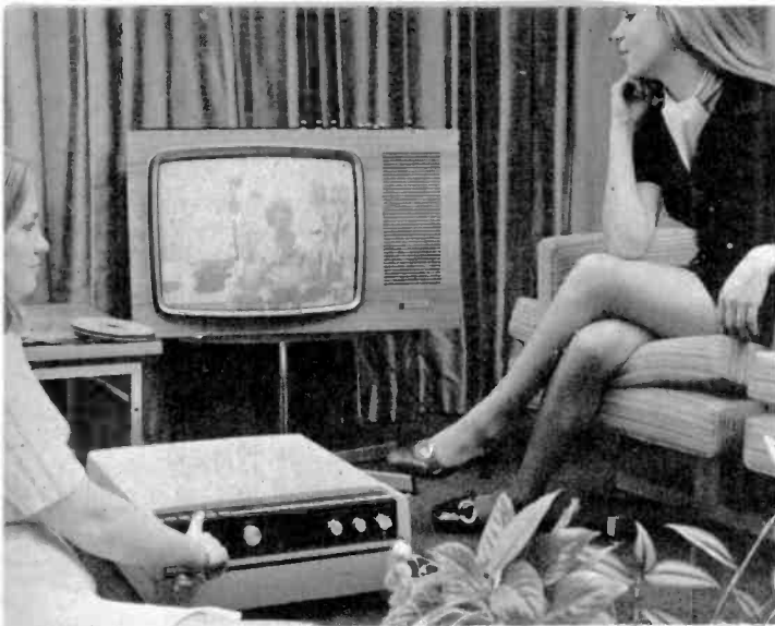
The EVR teleplayer can be connected directly to a domestic television set to provide pictures and sound from the telecartridge microfilm
