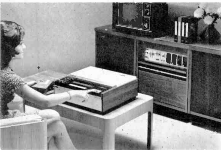
The Videocassette player connected to a colour television receiver. The tape can be stopped at any point in the programme, removed without rewinding and replaced with another cassette
