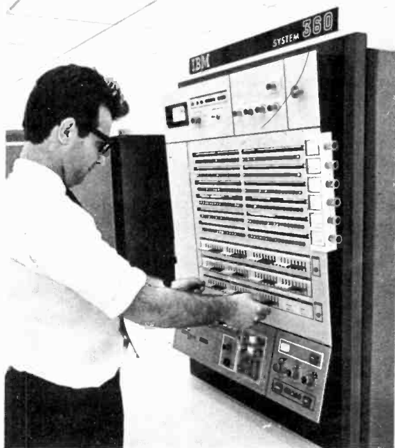
Magnetic data storage machines and information input and access points, in use inside the computer room, are shown above, whilst below an engineer is shown setting up one of the three IBM computers which form the main brain of BOADICEA
