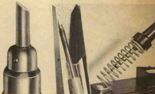
Fig. 2. The tip must be flat and tinned Fig. 3. Invest in a protective stand
