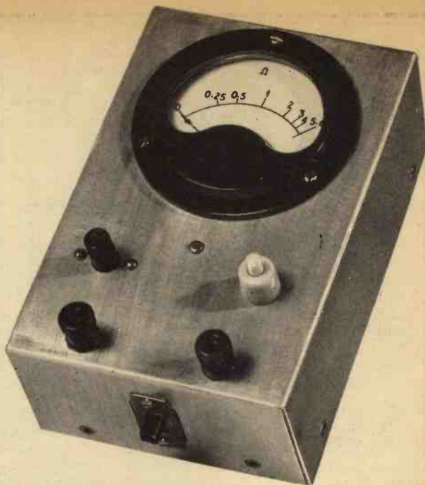
Front view of the ohmmeter clearly showing the new calibration of the dial
