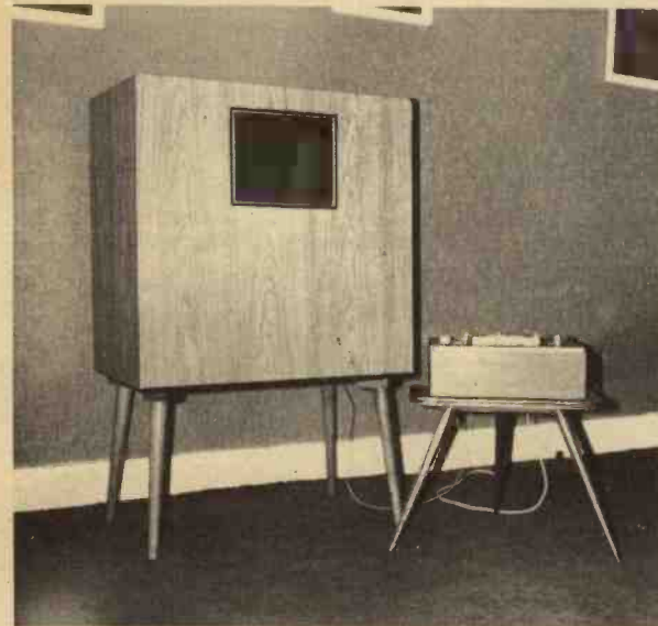
This photograph shows the new version c.r. colour pattern display based upon a discarded television receiver and which will be described in subsequent articles
