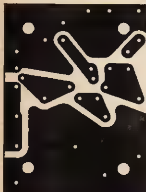
Fig. 3. Printed circuit pattern (full size) for the microphone amplifier
