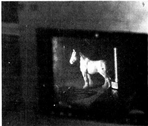
Fig. 2. Illumination of the hologram with red laser light gives a three-dimensional image lying behind the photographic plate
