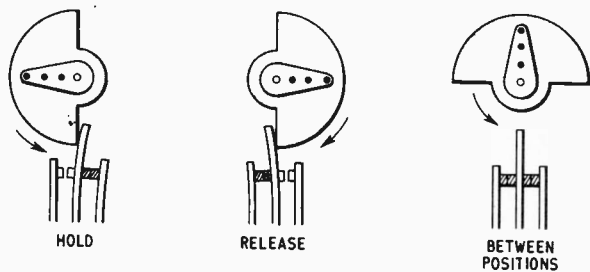
Fig. 10. Two-battery, two-position servo system
