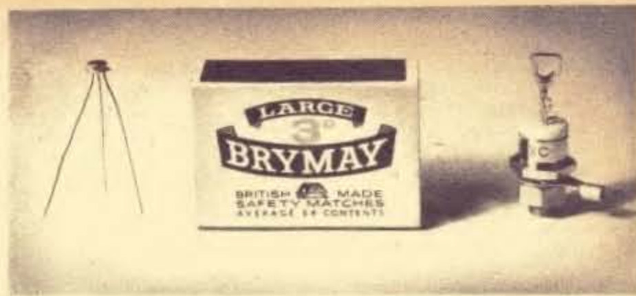
Size of a 200mA thyristor (left) and a 10A thyristor (right) compared with a matchbox
