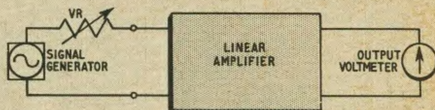
Fig. 3. Measuring the output of an amplifier to determine the 6dB voltage drop by adjusting the variable resistor VR
