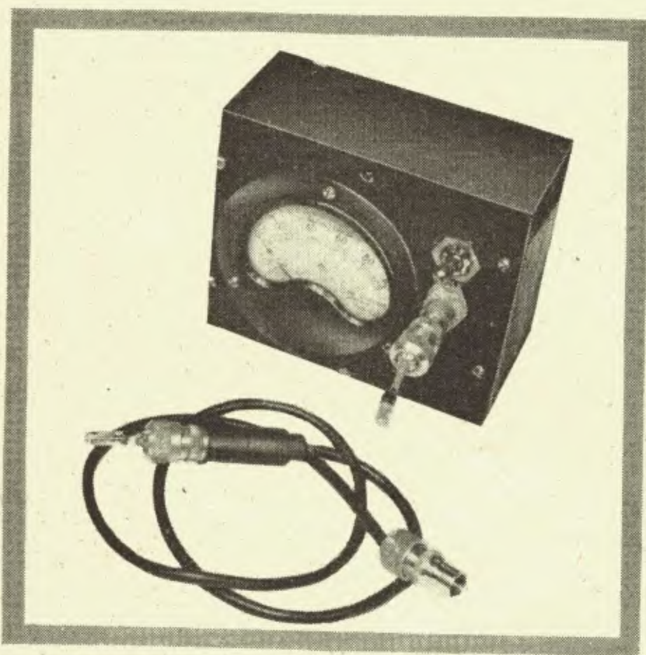
Fig. 1. Simple infra-red ray detector with probe attached. The extension lead with photocell probe is shown in the foreground
