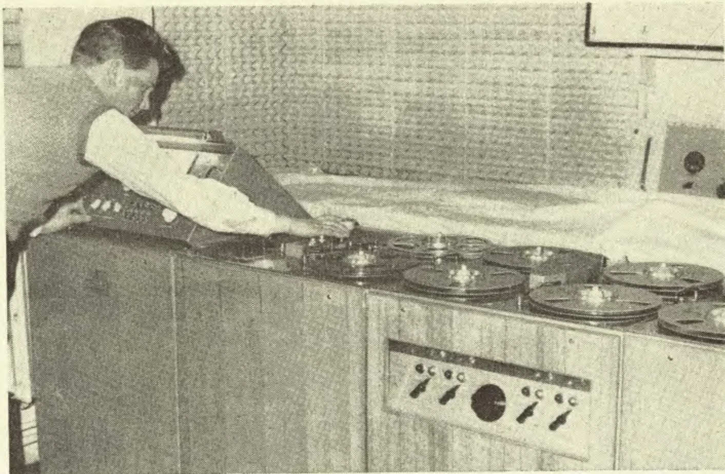
Fig. 3. Master tapes being reproduced at high speed from an original studio master on the left. The operator is speeding up the machine with an auto-transformer control. The recording equipment and the master copying equipment are at the head offices of the Royal National Institute for the Blind in Great Portland Street, London
