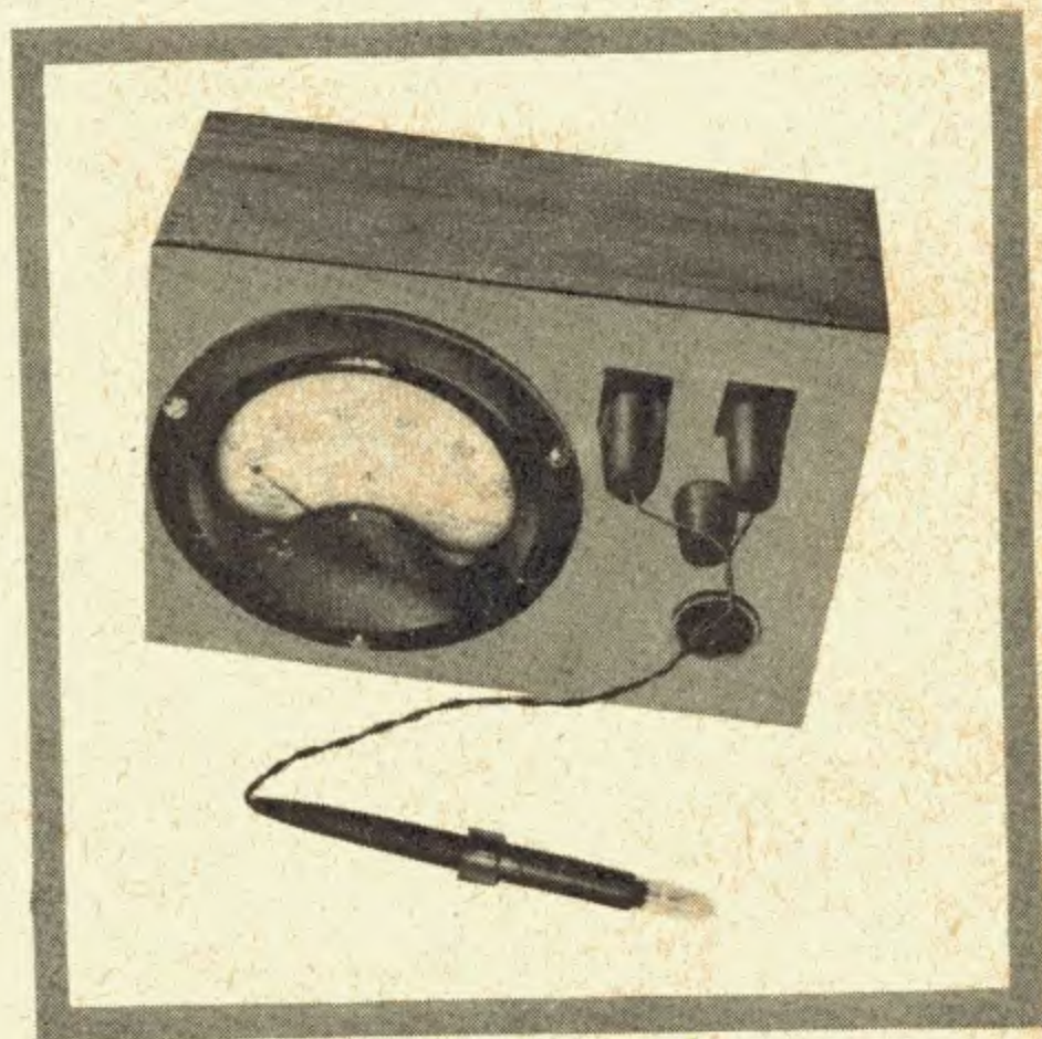
Fig. 6. Sensitive infra-red ray detector with probe connected by a twisted pair of wires and wander plugs
