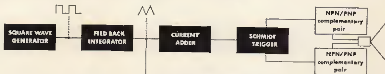
BLOCK DIAGRAM shows in simplified form the stages of function of this remarkable amplifier. Such design with its very much better standards of performance is made possible by use of the very latest in transistors and high quality components.
