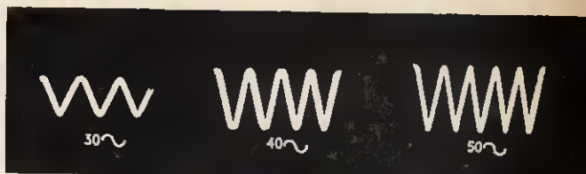
Fig. 3. Waveform of vent output in a 1 cu ft reflex enclosure fitted with an 8in unit and an input of 1 watt
