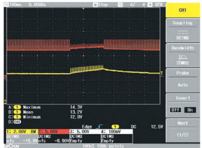
Fig.10: this shot shows the Charge Controller operation. The red trace is the 100Hz input from the charger, while the yellow trace shows the current into the battery.
