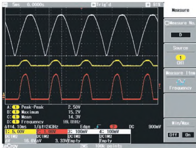
Fig.9: this scope shot duplicates the waveforms shown in Fig.2a. The white trace is the charger input, while the red trace shows the 100Hz current pulses into the battery.
