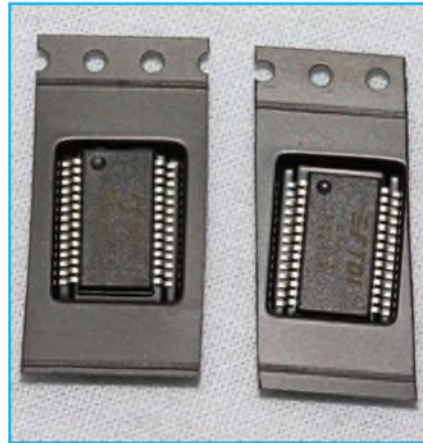
Fig.1. The FT232RL and FT245RL chips are surface-mount types that have 0.65mm pin spacing, and are tiny. The plastic case is fractionally more than 10mm long.
