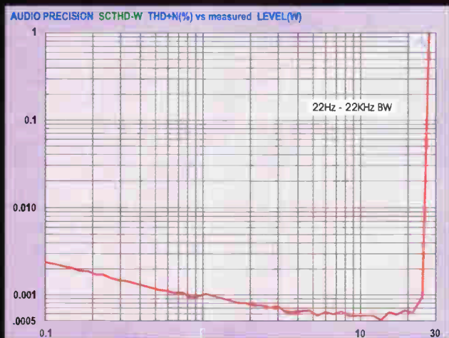
Fig. 1: this graph plots the total harmonic distortion (THD) at 1kHz from 100mW to just over 25W.
