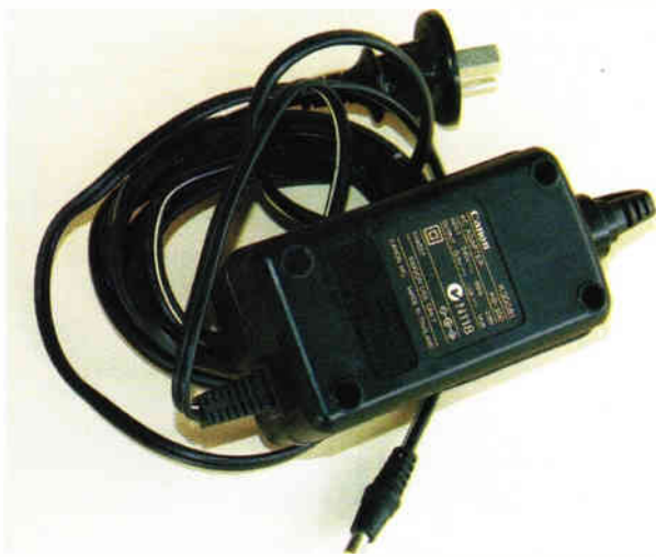
A 1A 13.5V plugpack makes an ideal foundation for a trickle battery charger. Plugpacks like this can be picked up for nearly nothing at the tip and where secondhand electrical goods are sold.
