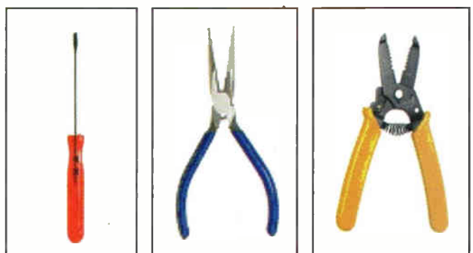
Fig.1.3: Three basic tools for assembling Protobloc projects: screwdriver, snipe-nose pliers and wire cutter/strippers
