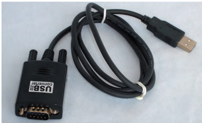
Fig.1. A USB-to-serial port converter looks like a simple lead, but there is some electronics in the serial port connector. It is powered from the USB port but there is no supply output on the serial port
