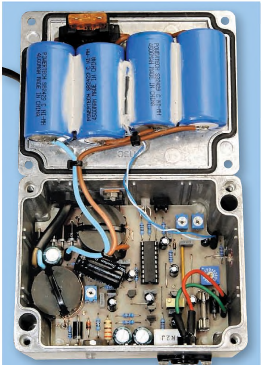
The High-Energy LED Lighting System is built into a rugged diecast aluminium box. It uses high-capacity C-size 4500mAh nickel metal hydride (NiMH) cells and can drive up to 6W of Luxeon LEDs. In addition, it has intelligent charge and discharge control and user-adjustable modes that allow it to be adapted to nearly any Luxeon LED lighting use.
