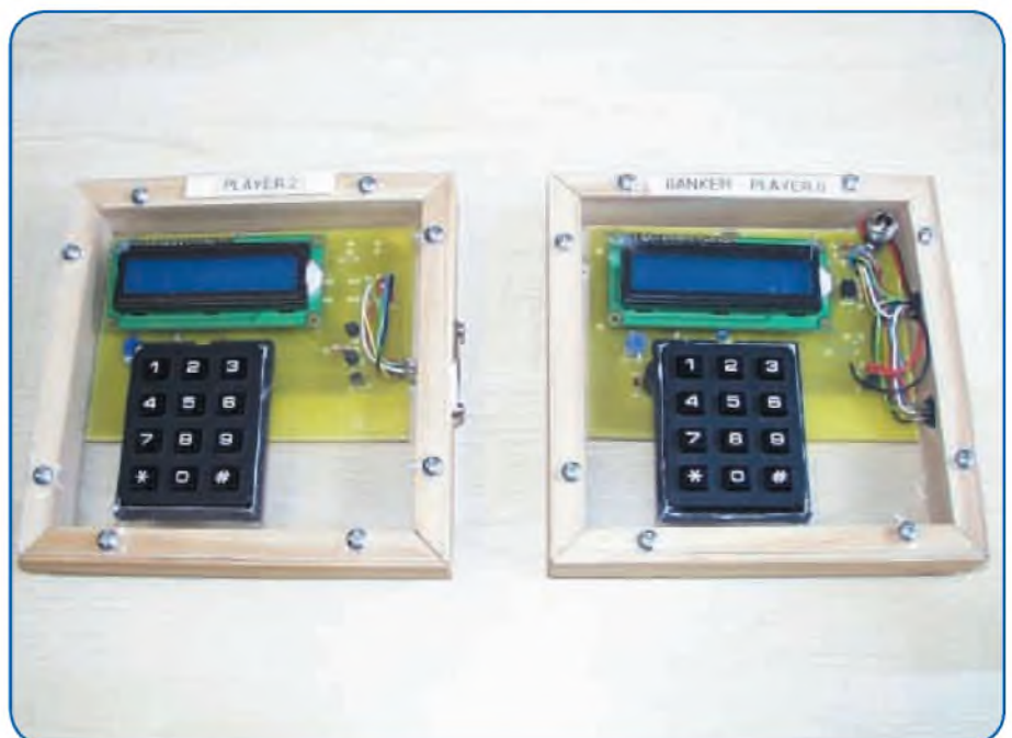
Prototype Player and Banker stations showing positioning of the keypads and the 16-character 2-line LCD modules. The DIN sockets are mounted on the sides
