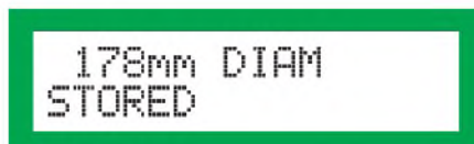
Fig.7: Confirmation of wheel diameter setting storage
