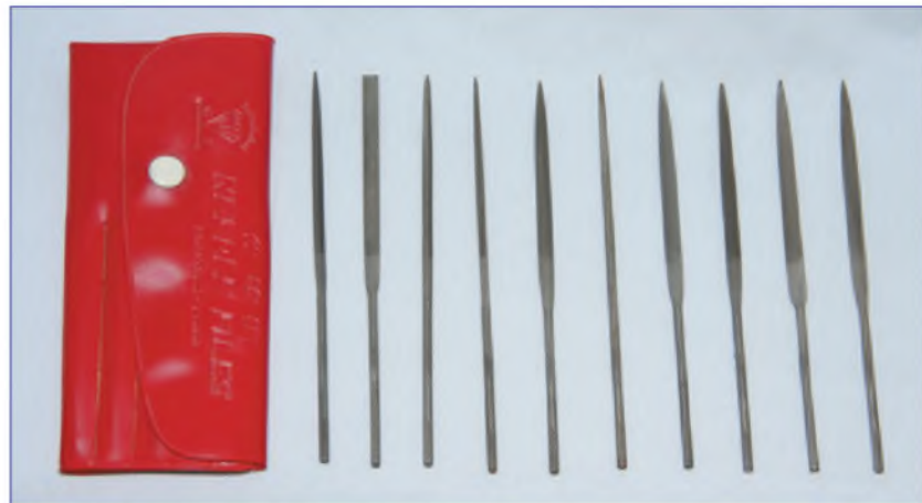
Fig.2. Needle files are often sold in sets containing a variety of shapes, but a round type is all that is needed for making cutouts. Other types can be used for tidying assorted holes.
