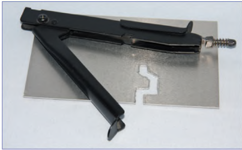
Fig.3. A hand nibbler can quickly cut through most thin sheet materials. A tool of this type is best suited to large cutouts having straight sides
