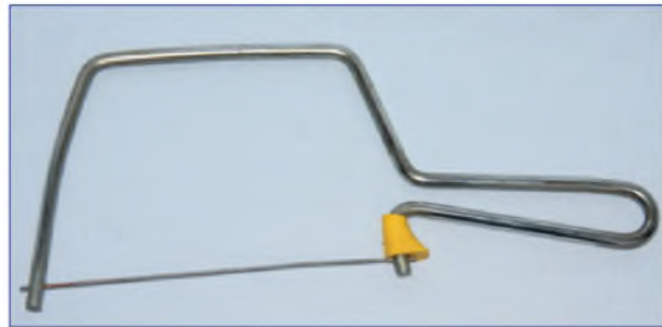
Fig.1. A coping saw is relatively inexpensive, but can be used to make cutouts of practically any size or shape. With practice, it is possible to produce very accurate results
