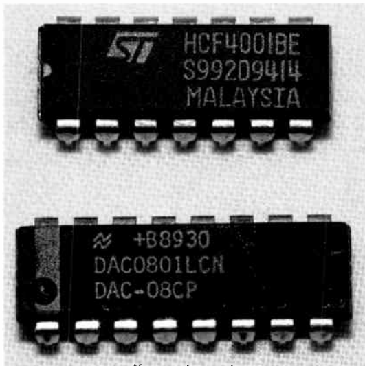
Fig.2. Most semiconductors have extraneous markings. These two chips are a CMOS 4001B (top) and a DAC0801LCN digital-to-analogue converter chip
