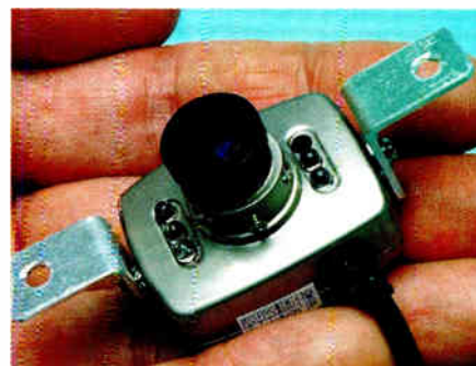
The Video Reading Aid is based on a miniature black and white CMOS camera, such as this Swann unit.
