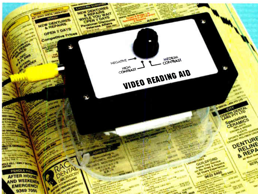
The Video Reading Aid skates over the printed page on a plastic skirt (actually an upside down food container). This keeps the lens at the correct focal distance and makes the unit easy to operate.
