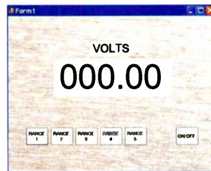
Fig.5. In this example the background is provided by a photograph of an aluminium panel. Any bitmap in JPG, GIF or BMP format can be added to the form
