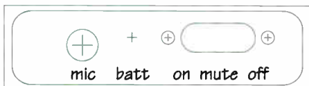
Fig.5: this artwork can be used as a drilling template for the front panel.
