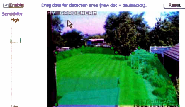
Defining the area to be triggered by CAM Wizard motion detecting software. The tree has been excluded to prevent nuisance triggering
