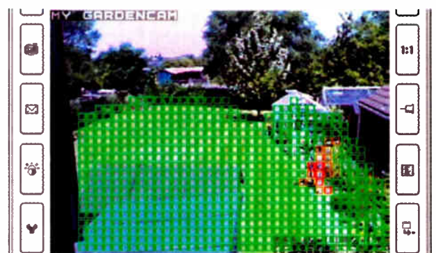
Motion detected (red highlights) in the area being monitored (green squares) triggers the alarm
