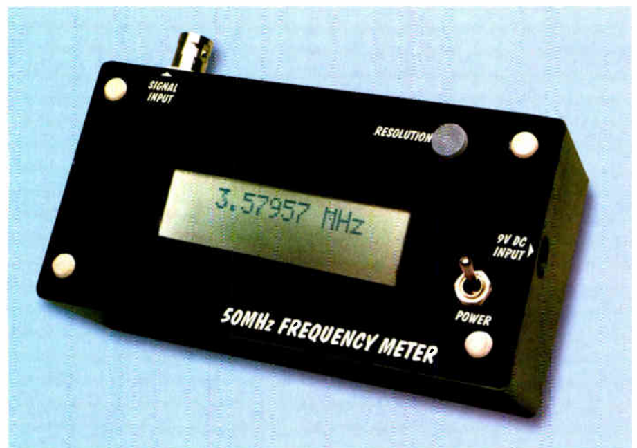
This photo clearly shows the location of the access hole for the DC input socket for Version 1. It's located on the opposite side of the case for Versions 2 and 3.
