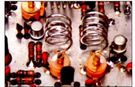
Photo 11.1. Coupled tuned circuits in the RF amplifier stage of a VHF receiver
