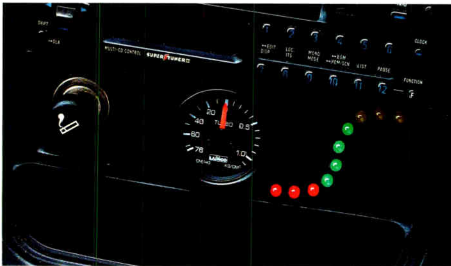
In this installation, round LEDs have been used for the mixture display, mounted remotely from the PC board. Note how the owner has chosen to arrange the LEDs to mimic the response curve of the sensor. This is a great approach if there is sufficient room available. [Michael Knowling]
