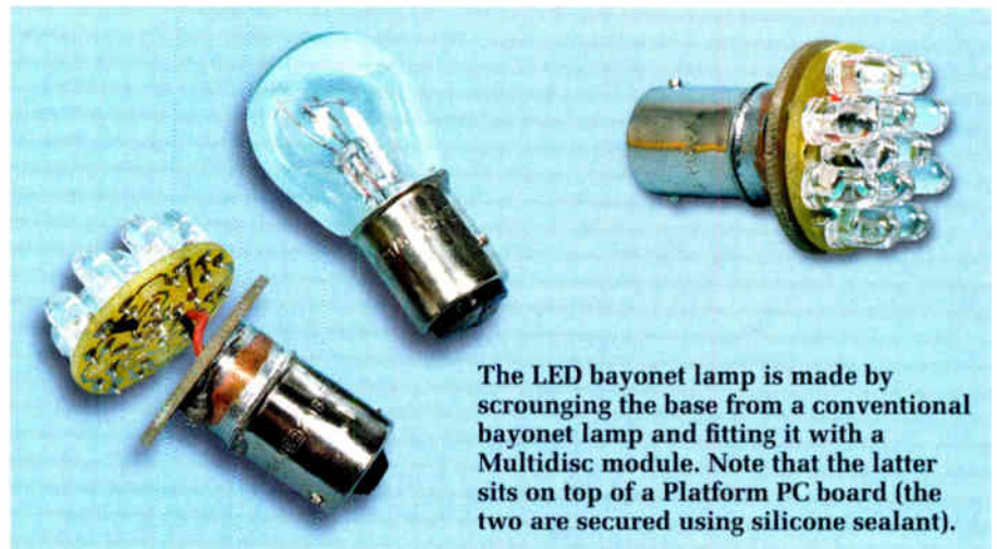
Fig.6: follow this diagram and the step-by-step instructions in the text to make the Bayonet lamp assembly. The Multidisc assembly can be fixed in place with silicone sealant.
