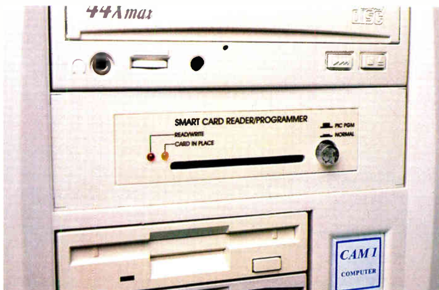
We fitted our prototype to a standard 3.5-inch to 5.25-inch drive mounting kit which was then slotted into a spare drive bay.
