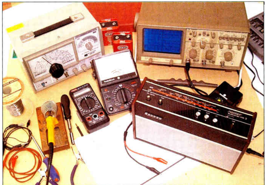
Photo.7.1. A selection of typical bench test instruments including a signal generator, digital and analogue multimeters, and an oscilloscope
