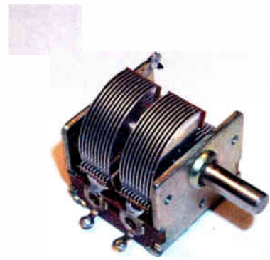
Photo 3.3. An airspaced variable capacitor used for tuning a radio receiver. This component is a dual-gang type that has two separate sections, each of which is variable over the range 5pF to 365pF
