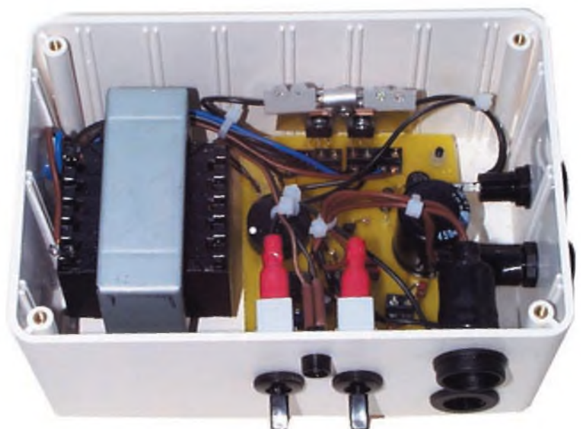
General layout of components inside the plastic case. The mains transformer tags must be covered and positioned close to the sidewall of the case.
