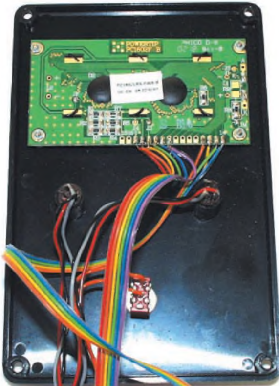
Rear of the case lid showing the l.c.d. module and wiring to the three switches.
