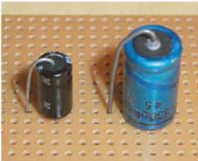
Fig.3. Mounting axial components vertically is best avoided but is called for by some component layouts. As usual, mount the components with the bodies as close to the board as possible.
