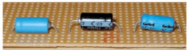
Fig.2. Components should be mounted flush with the surface of the board (left) and not with a gap underneath (centre and right).
