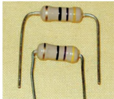
Fig.1. The leads are normally formed a millimetre or two from the body (top) and not right next to it (bottom).
