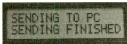
Example display when downloading stored data to a PC-compatible computer has been completed.
