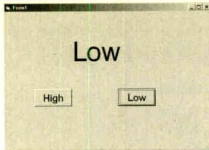
Fig.3. The modified program will read back the level set on the TXD output line.
