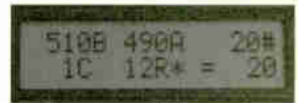
Example display when carrying out soil monitoring with S9 switched on to test mode.
