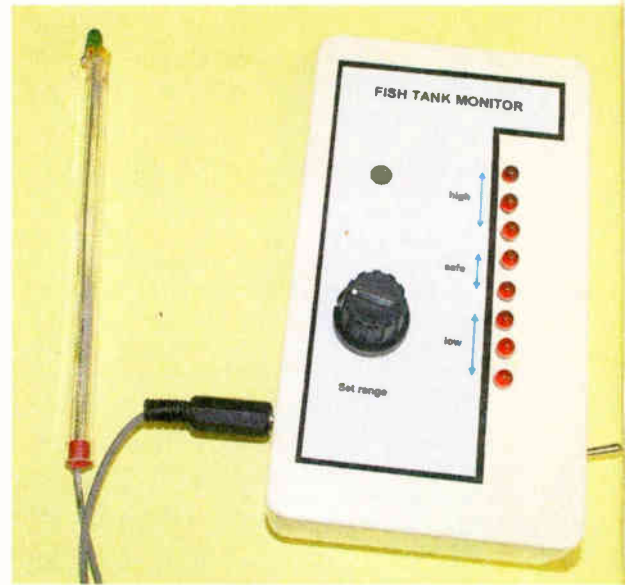
Completed Temperature Sensor module. Note the thermistor mounted in a discarded ballpoint pen barrel.
