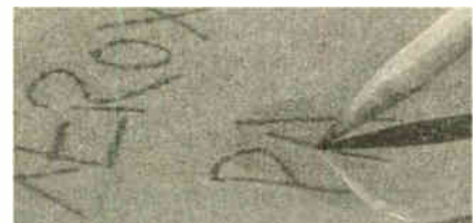
An electronically charged pencil rotates the bichromal beads in a sheet of Xerox electronic reusable paper.
