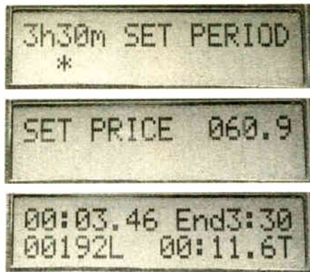
Example displays: Setting water flow duration period; setting price per cubic metre; during monitoring.
