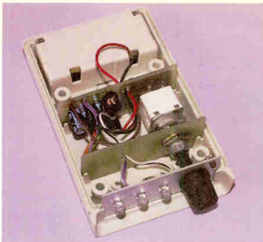
Completed White L.E.D. Super Torch. Note the 3mm "low battery" monitor l.e.d. in the top right-hand corner of the front panel.
