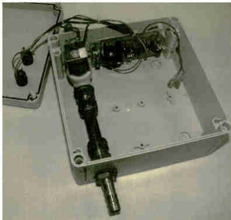
Layout of components inside the completed unit. The large "empty" area is reserved for the sealed lead-acid battery.
