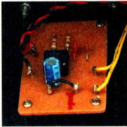
Audio Alarm p.c.b. Note the wire link replacing resistor R4.
