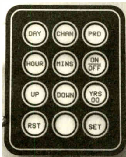
Photo 2. A 3 x 4 self-adhesive membrane keypad. The legends can be customised using "slide-in" tabs.
