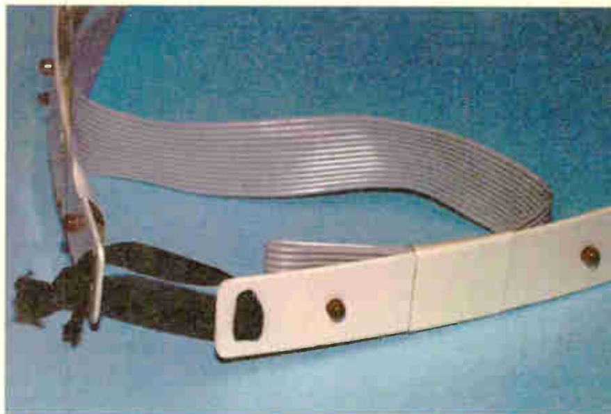
The two ends of the I.e.d. carrying plastic strip are secured with elastic to form a headband, hatband, belt etc: Take your PIC!
