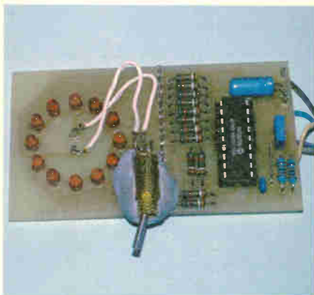
Programming switch soldered to the "link" pins on the p.c.b.
