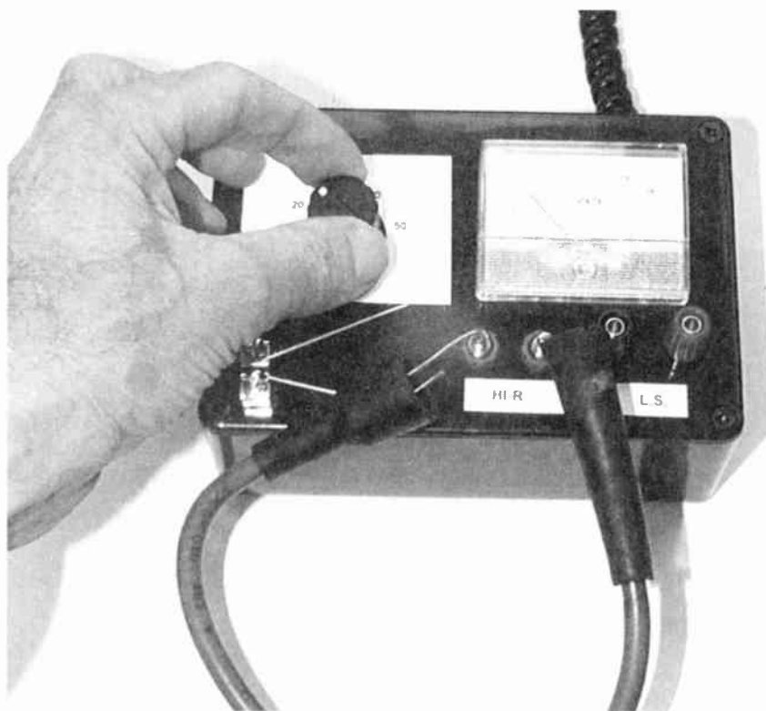
Testing an ignition (plug) lead. The new meter scaling can also be seen here.
