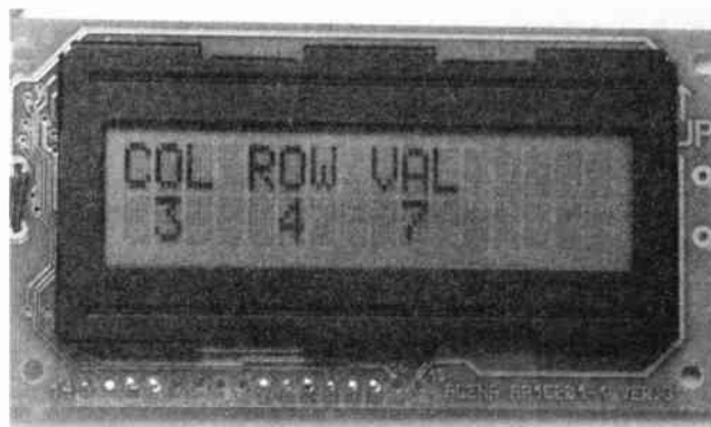
Photo 12.7. Typical alphanumeric l.c.d. screen. This one has two lines, each of 16 character cells.
