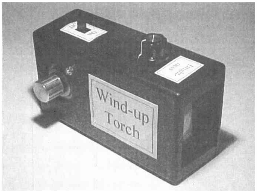
Completed Wind-up Torch showing the small wind-up knob and l.e.d. lens beam window.
