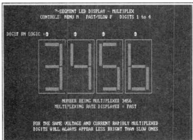
Photo 12.4. Screen dump of the interactive 4-digit l.e.d. display being multiplexed at a fast rate, all digits appear visible.
