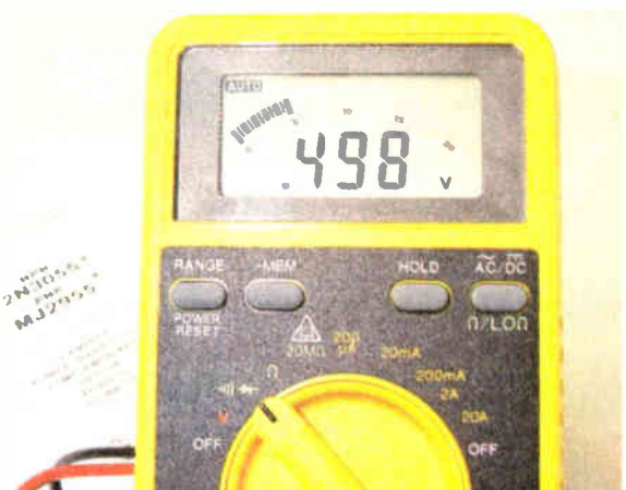
The diode test range of a digital multimeter can be used to measure the forward voltage of a transistor diode. A good reading is in the region of 0.45V to 0.9V.
